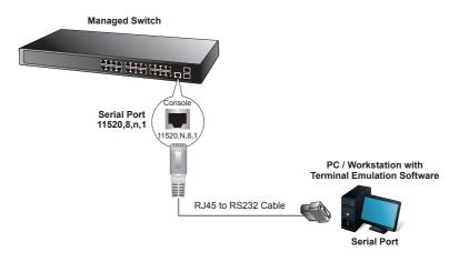
Figure 3-1: Managed Switch Console Connectivity
